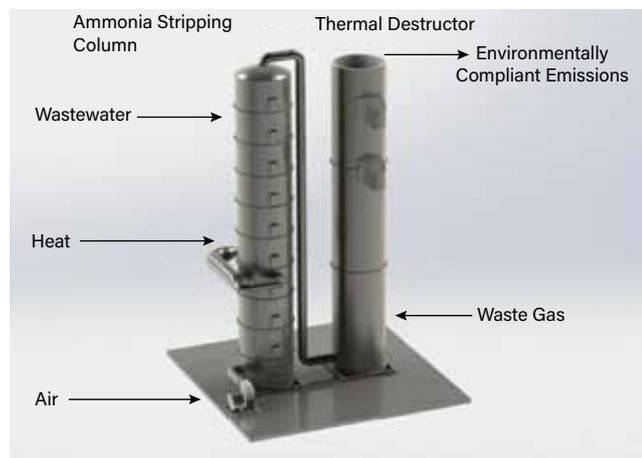
▲ **Figure 6.** A thermal ammonia stripper uses heat to remove ammonia from a wastewater stream.
